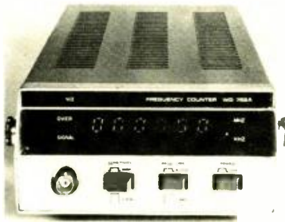
The counter operates on 115V ± 10V 50 60 Hz. The unit measures only 2 5 / 8 by 5 3 / 4 by 9 1 / 4
