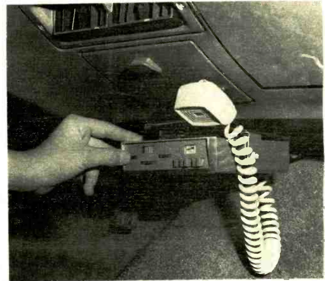
FIG. 8—MICROPHONE BRACKET should be mounted so that the microphone cable does not interfere with the driver's foot.
