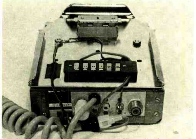
FIG. 4—RELIABLE CONNECTIONS are attained by unsoldering the wires supplied with the slide mount and soldering the wires from the transceiver directly to the terminals on the slide mount.
