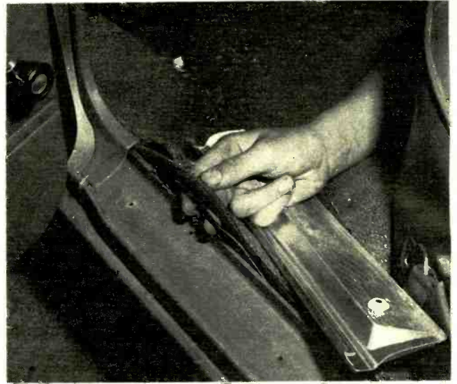
FIG. 6—TRANSMISSION LINE is run from trunk to passenger compartment in wiring-channel under the door saddle.
